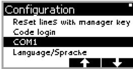
On the one hand, the use is determined, on the other, the baud rate of the interface can be set.
