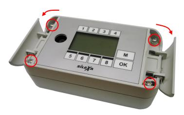
After this you can lift the top part and open the housing.
