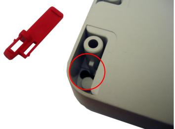
The sealing pin can then be fixed with a special cable tie or a lead seal, so the housing can not be opened undetected. A second sealing pin can be used on the opposite side.
