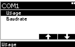
The COM1 port can be used as a printer interface. The buttons and select the function, while confirming with OK. M cancels the selection. If the printer is active, then in the evaluation there is the possibility to print on the external printer. By default, the COM1 port has no fixed use.
